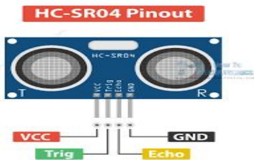
Ultrasonic sensor HC-Sr04
