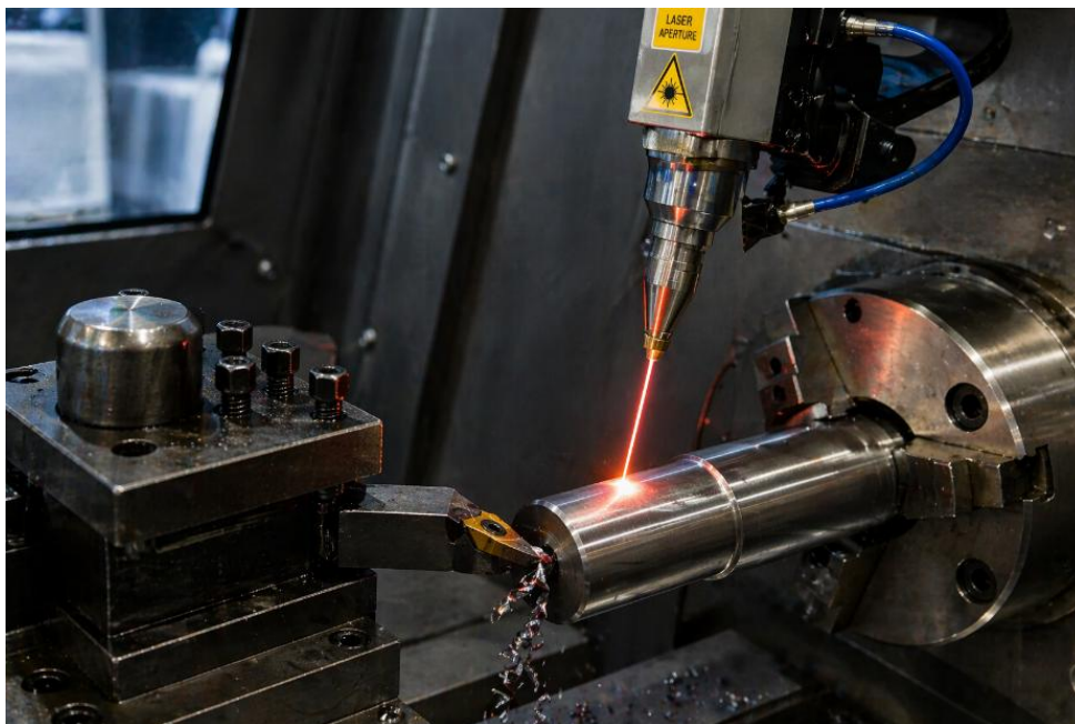
Figure 1 — Schematic of laser-assisted machining process
